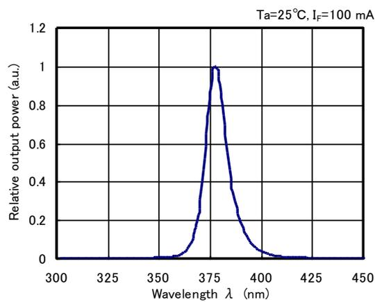
Optical and electrical characteristics depend on packaging method. The above data is for SMD packaged LED.
